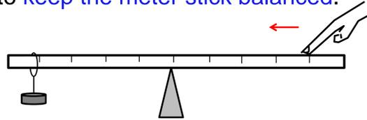
2. Slide fingers along the meter stick to locate the balance point, or Center of Gravity (CoG), of the meter stick.
