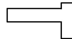
4. Students are asked to draw a line to divide the "T" into two rectangles, and to draw two dots to represent the CoG of each rectangle. Again predict the CoG of the "T".
