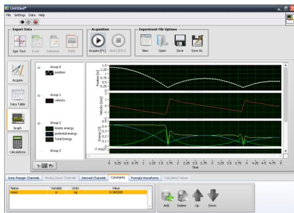
**FIGURE 2.** Data acquisition user interface. Buttons across the top are data acquisition and different file functions. Tabs down the left side control which graphs or data tables are displayed in the central area. In the lower panel the user defines data acquisition channels, calculation constants, derived and calculated data sets and statistics to calculate.
