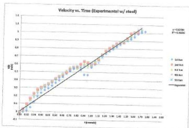
The velocity v. time graphs are much more interesting. Between approx 0.8 and 0.9 s, there is clearly an anomaly in the data. This is likely the fault of the table.
