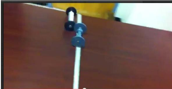
Roller C wins by about a wheel diameter...note that it has more of its relative mass near its axis of rotation (because the axle is made of aluminum rather than plastic)
