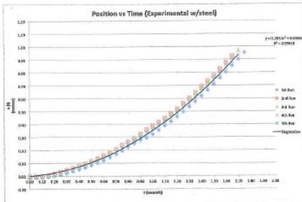
The position v. time graphs are very close to the theoretical graph. At the max  $x$  value on the graph ( $x=2$ ) the largest discrepancy should be present as the value is ignored. All values are w/in 0.1 second of one another from both exp. graphs and the theoretical.
