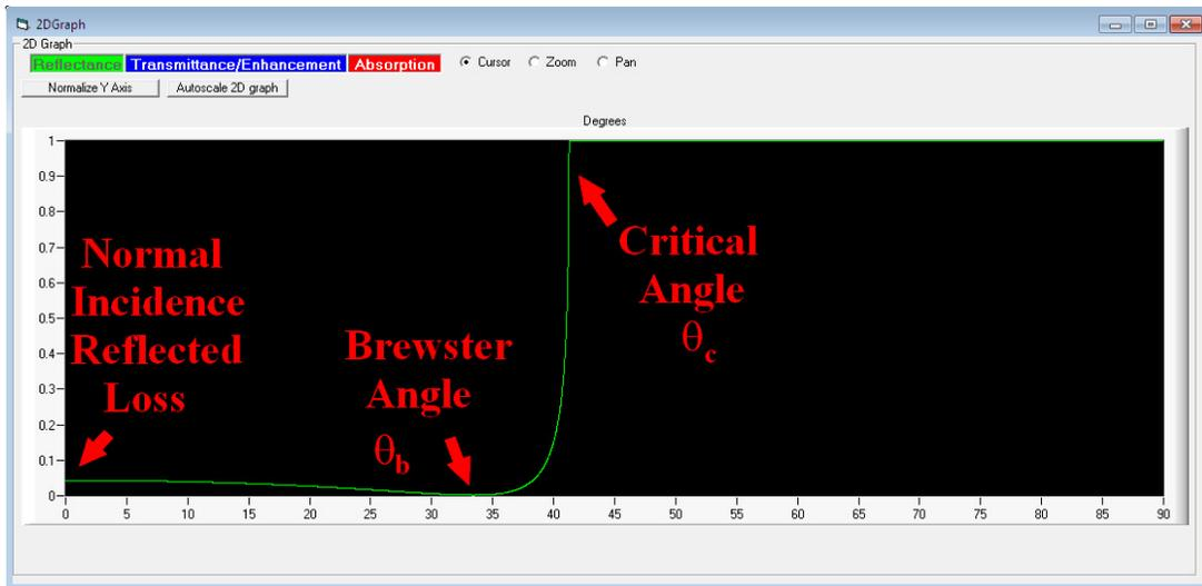
**Figure 5**, Theoretical modeling with Fresnel equations of Reflectance-vs-Incident angle. Three distinct regions are of importance; the normal reflection from an interface at normal incidence (glare), the angle with the minimal reflection of light (Brewster angle), and the point whereby any light after the angle gets totally reflected (Critical angle).
