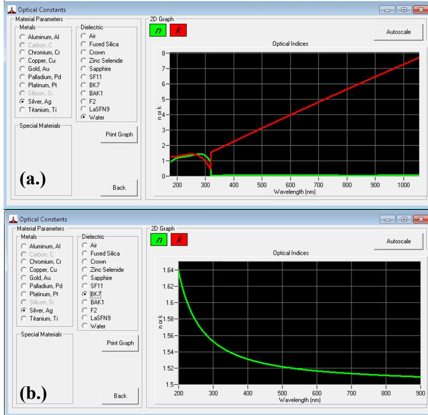
**Figure 1**, Optical constants,  $n$  and  $k$  ,for (a.) silver (Ag) and (b.) optical glass (BK7). Green denotes the real part of the complex index,  $n$  and red indicates the extinction coefficient,  $k$ .
