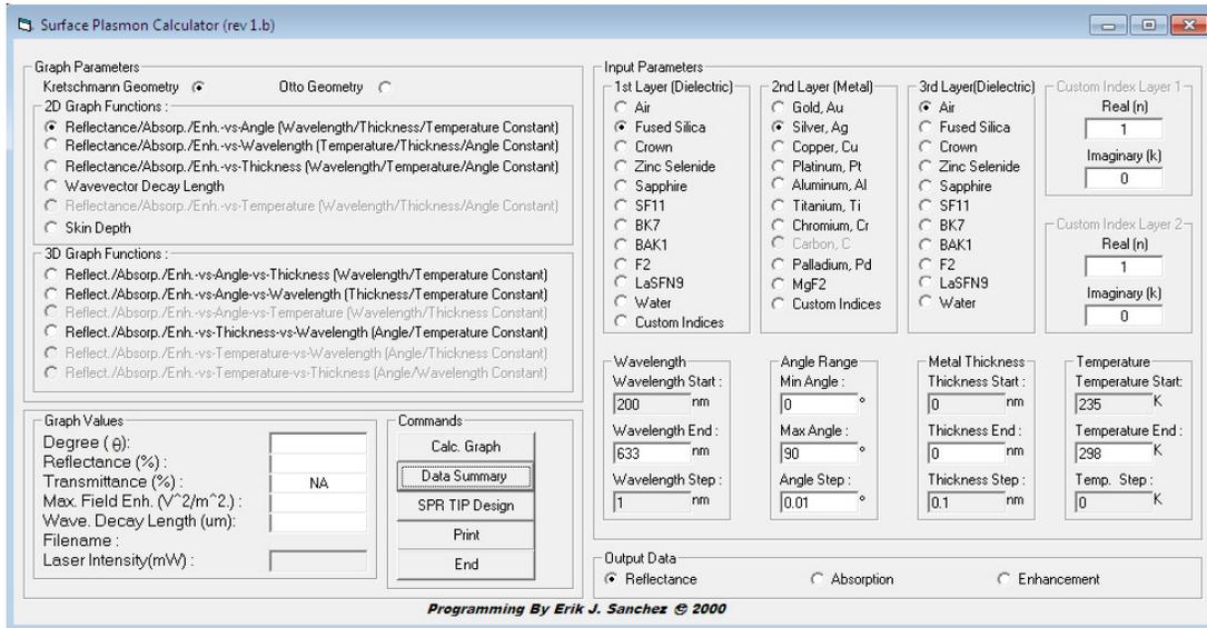
**Figure 4**, Example of the author's GUI, although this is very user friendly, any version including text would do the job. The user can choose 2D or 3D configurations as well as Kretschmann-Raether or Otto configurations for modeling. The custom indexes can be used for a specific material which is not in the database.
