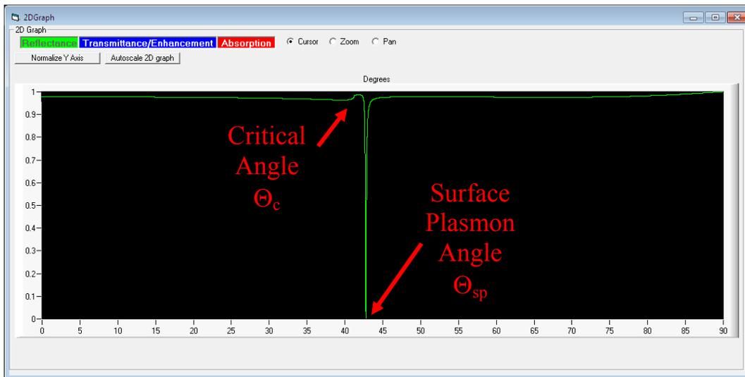
**Figure 7**, The Modeling of Fresnel equations to demonstrate the Surface plasmon resonance of a BK7 prism, Ag of an undetermined amount and Air as a three layer system. The level of resonance is oftentimes given as the narrowness and depth of the dip after the critical angle. The reflectance can be as low as  $1 \times 10^{-7} \%$ .
