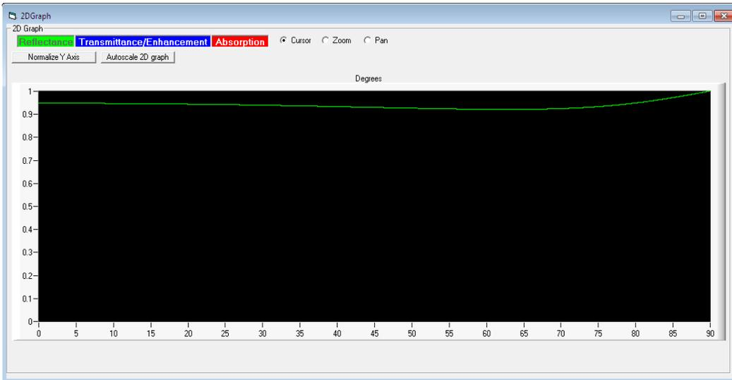
**Figure 6**, A theoretical modeling using Fresnel Equations of 300 nm of Ag on a BK7 prism as a function of incident angle. For the most part the light just reflects back as expected.
