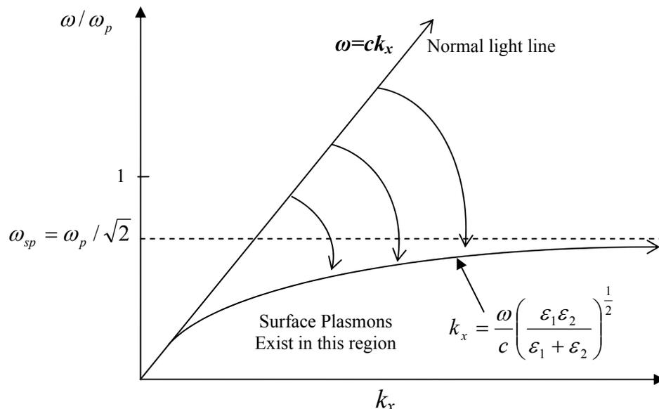
**Figure 2**, Dispersion relation, frequency,  $\omega$  versus wavevector magnitude,  $k_x$  of the surface wave in the x direction. The surface plasmons exist in the region where the wavevector is larger than in the incoming incident field, since the permittivities have just the right values, the light line moves down.
