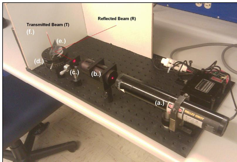
**Figure 9**, SPR optical experimental setup. (a.) Polarized HeNe 633 nm laser, (b.) beam expander, (c.) slit on a linear translator, (d.)
