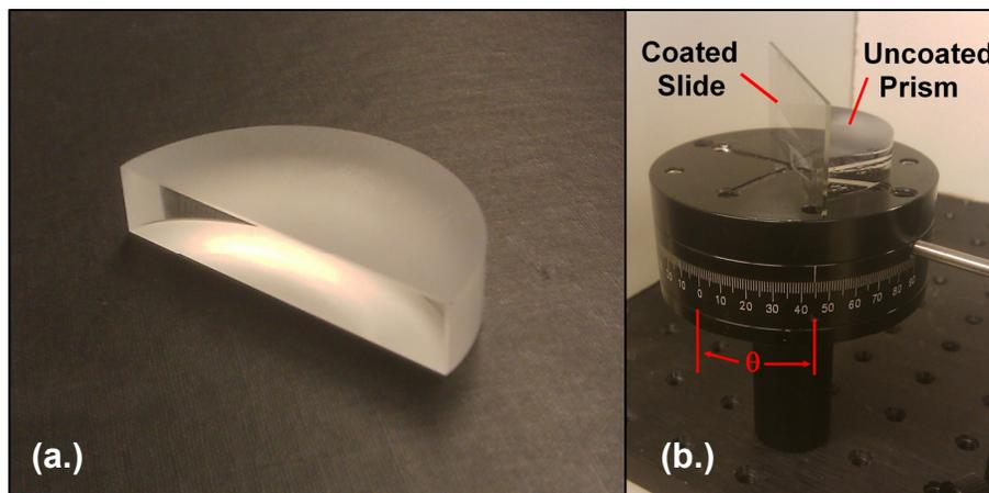
**Figure 10**, (a.) Optical glass prism used in the SPR setup, (b.) the optical rotator which holds the prism and can easily be read when it is rotated.
