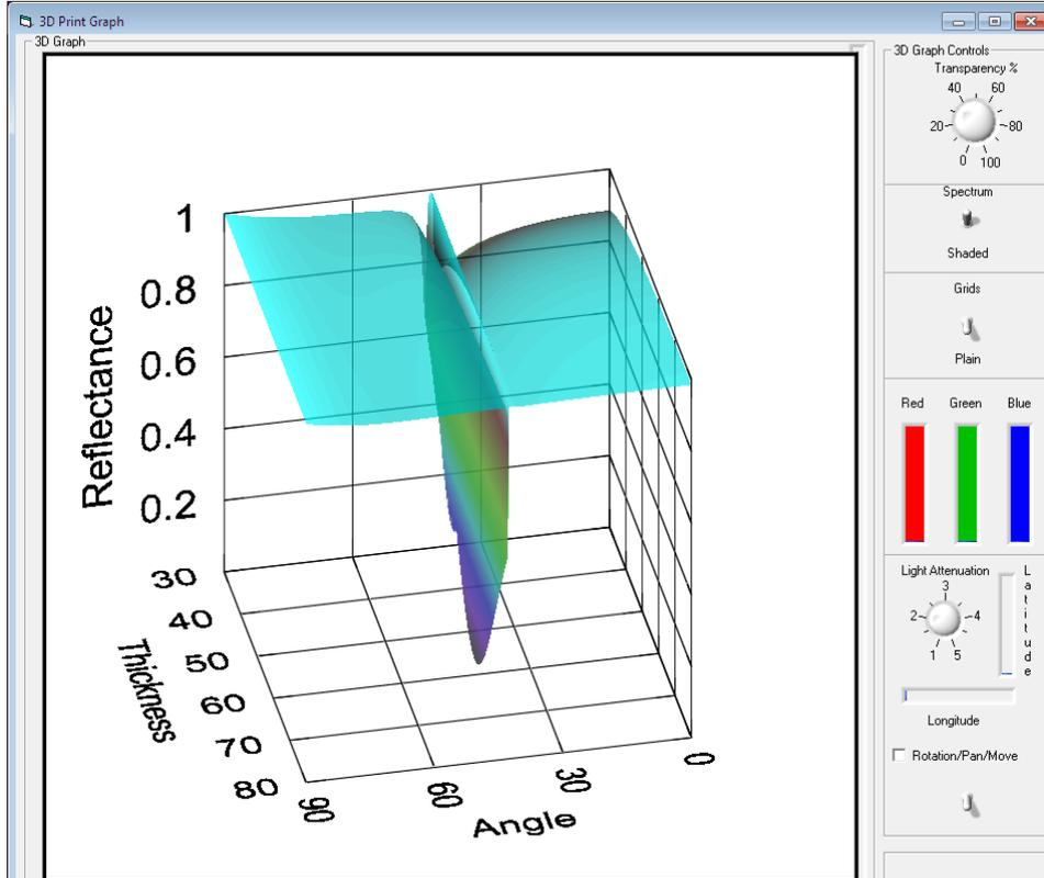
**Figure 8**, 3D modeling of the Fresnel equations for determining Reflectance as a function of Thickness of metal coating and Incident angle.
