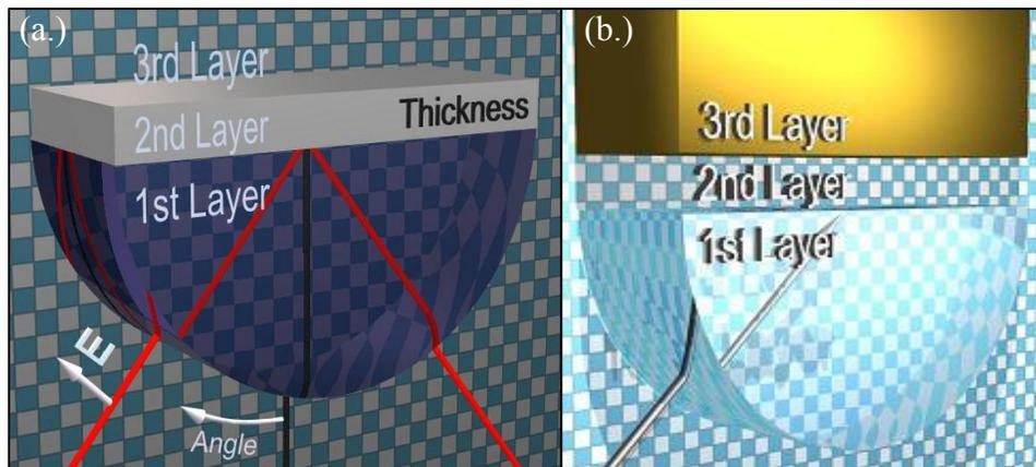
**Figure 3**, Two examples of Attenuated Total Reflection (ATR) SPR measuring techniques, the (a.) Krestchmann-Raether geometry and (b.) Otto Geometry.
