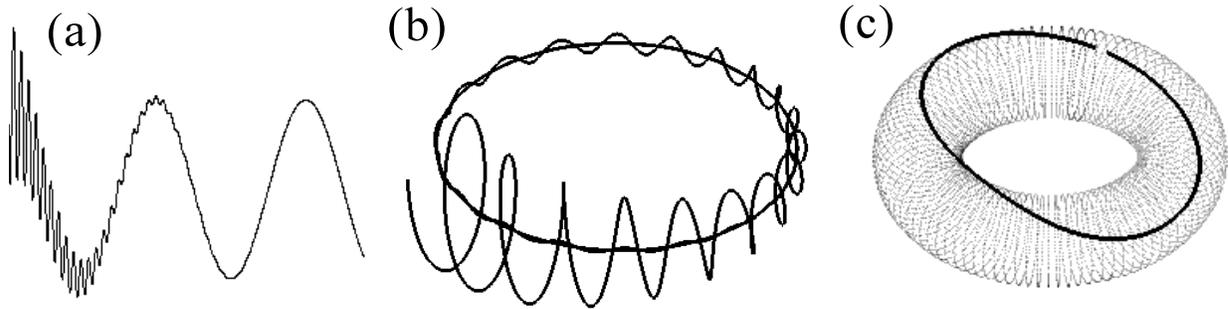
Figure 5: (a)  $\theta$  vs.  $t$  for a linear oscillator. (b) The same data represented as a phase space trajectory. (c) The dark curve represents the steady state trajectory (attractor) for a linear oscillator. It lies on a torus.
