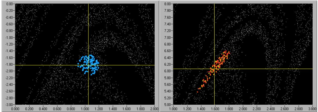
Figure 8: A small area of a Poincaré section showing how an initial set of  $\delta \mathbf{u}_n$  around the cursor in the left plot move and change shape when propagated 1/5 period. The scale ranges are the same in the two figures and the evolved set  $\delta \mathbf{u}_{n+1}$  is the elongated and flattened patch around the cursor in the right figure.
