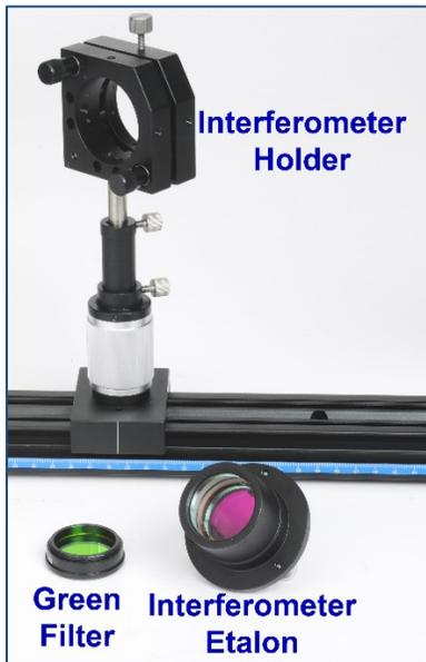
Figure 14: Filter and Interferometer
