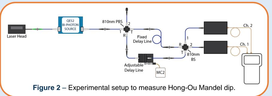
Figure 2 – Experimental setup to measure Hong-Ou-Mandel dip.
