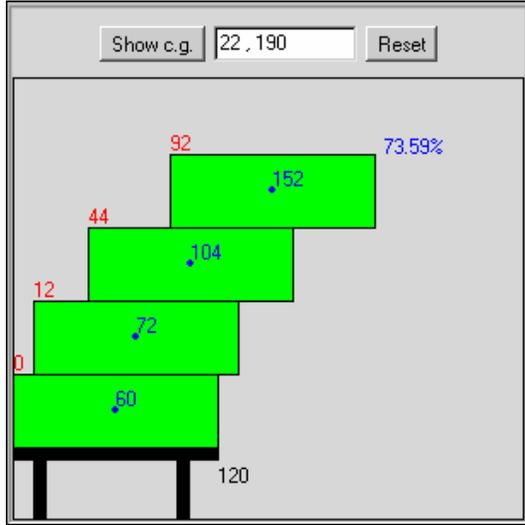
How can you stack four uniform bricks (or blocks or meter sticks) one on top of another so that they extend as far over a table as possible and yet remain stable?
