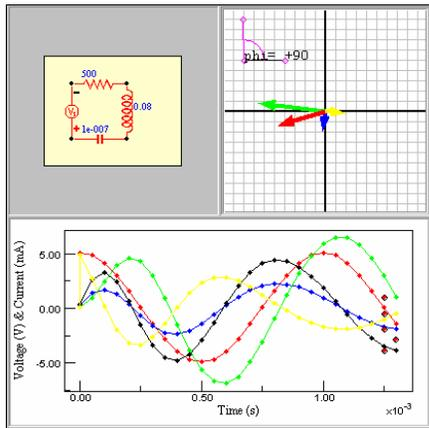
Assume an ideal power supply. The graph shows the voltage as a function of time across the source (**red**), the resistor (**blue**), the capacitor (**green**) and the inductor (**yellow**), as well as the current through the circuit (**black**) (voltage is given in volts, current is given in milliamperes, angles are given in degrees, and time is given in seconds). [Restart](#).
