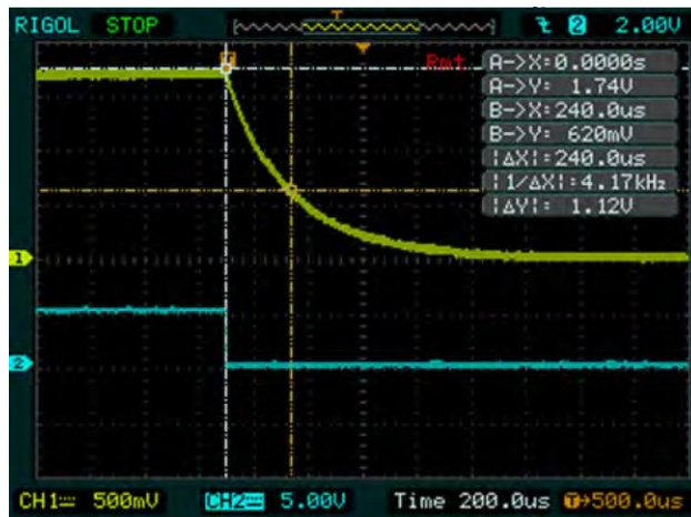
Figure 18, Fluorescence lifetime decay for Nd:YAG, similar but longer than Nd:YVO 4 .(Ref. 6)
