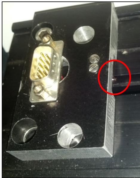
Figure 21 , Image of interlock unit for safety. The red circle indicates the limit switch which is connected to the DB-9 connector. If the laser unit is not pressed up against this unit, the laser shuts off.
