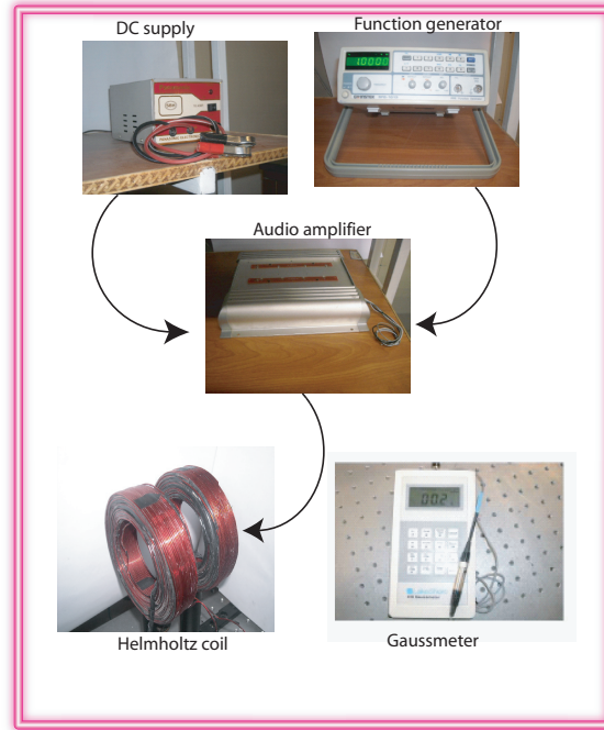
Figure 14: Instruments for creating and detecting the oscillating magnetic field.
