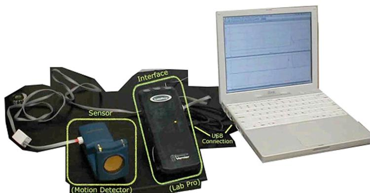
Figure 2: Technology setup consisting of sensor, interface and laptop computer connected via USB connection
