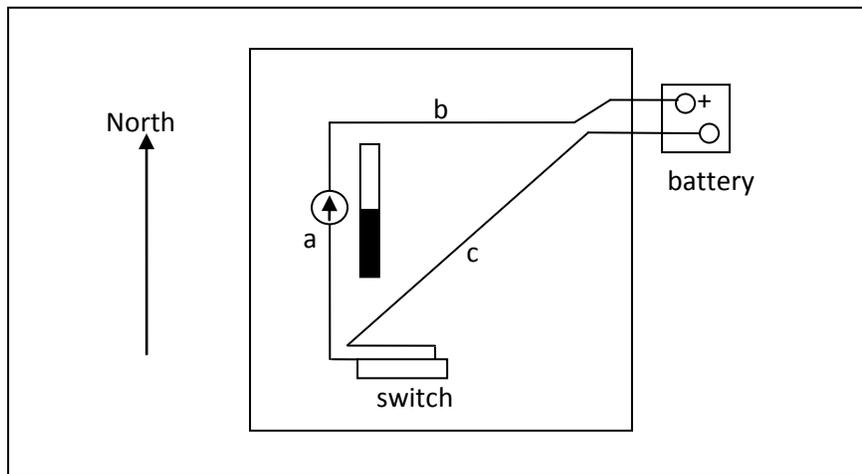
4.2 "Apparatus" set up. The compass is the circle with the arrow in it above wire "a" and a bar magnet is placed parallel to the wire, centered on the compass. The bar magnet's South pole is shown in white and the North pole in black.
