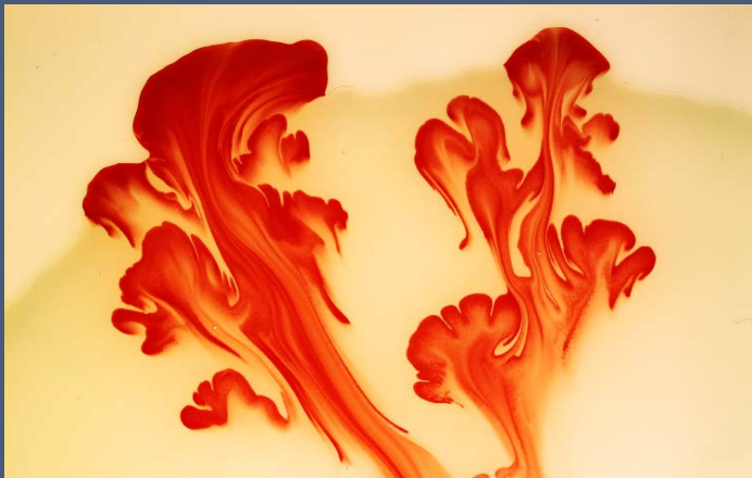
Above: Saffman-Taylor instability in a Hele-Shaw cell: dyed water injected into honey. Travis Ochsen, Grant Meaux, Shane Weigel 2011 Right: Only one 'bathtub vortex' formed in a bucket with two holes in the bottom, viewed from the top with food dye. Jonathan Varkovitzky, Chris Svedman, Peter Mitrano, 2010. Far right: Dyed mineral oil, illuminated in the UV, forms vortex rings upon injection by syringe. Jacob Varhus, 2013.
