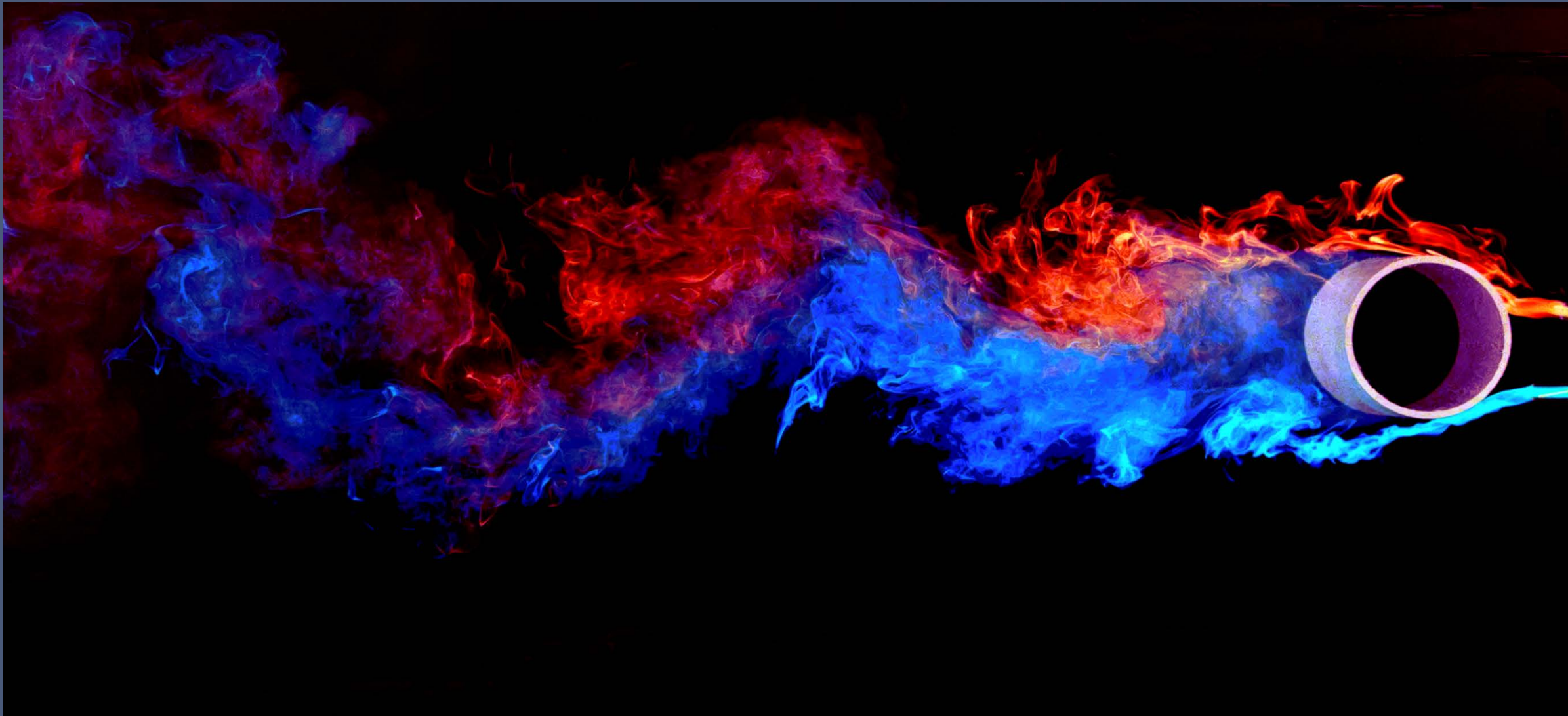
Turbulent flow in a flume around an obstacle, visualized with dye, and color-reversed. Kyle Manhart, Gregory Kana, Jared Hansford, Matthew Campbell, Andrew Scholbrock, 2011.
