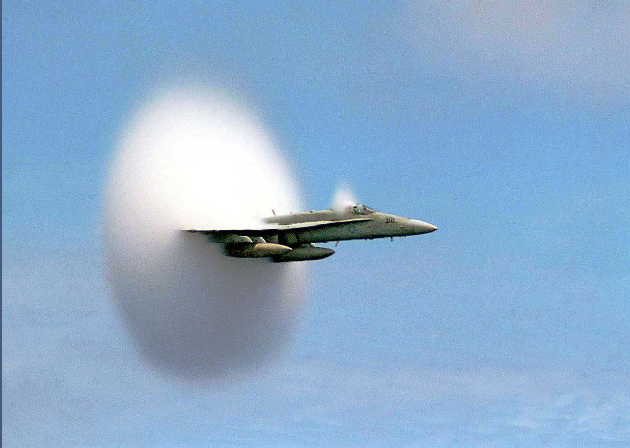
FA-18 Hornet breaking sound barrier. U.S. Navy photo by Ensign John Gay, 1999. Temperature drops in the expansion wave behind the attached shock, resulting in condensation. http://www.news.navy.mil/management/photodb/photos/990707-N-6483G-001.jpg
