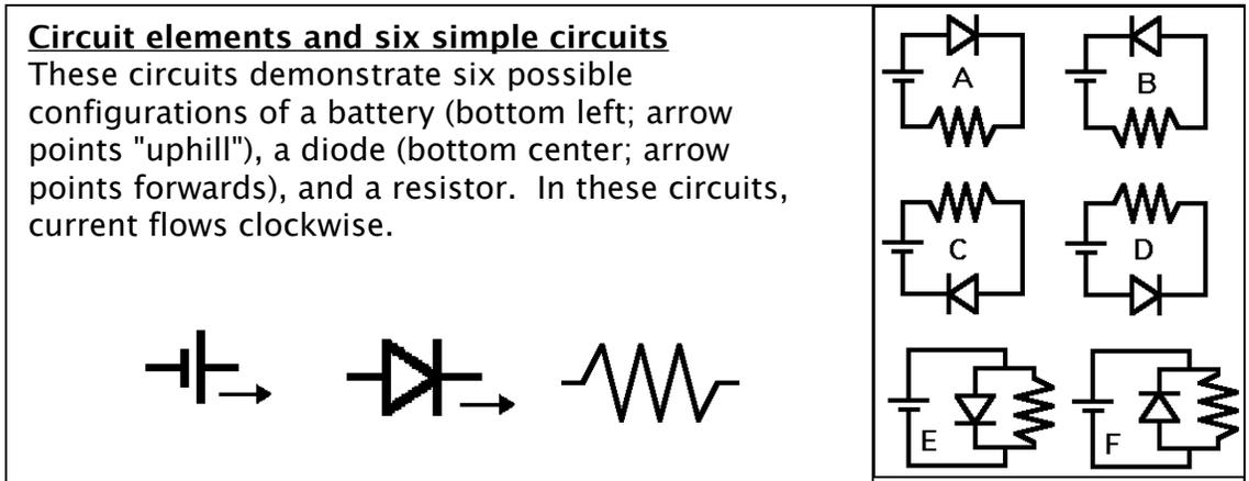
**Figure 6. Circuit Elements and six simple circuits**
