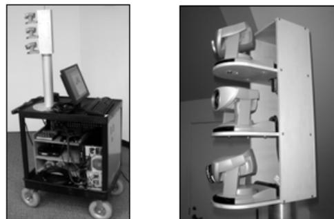
**FIGURE 1.** MScribe recording cart and camera stalk.
