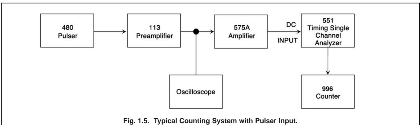
Fig. 1.5. Typical Counting System with Pulser Input.
