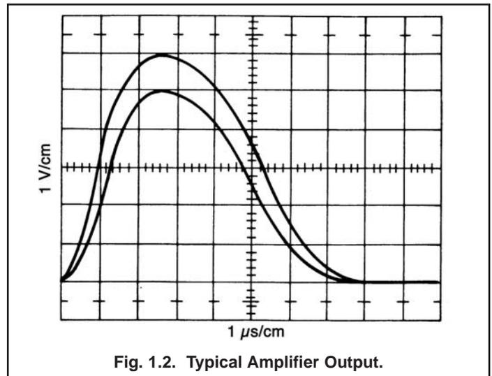
Fig. 1.2. Typical Amplifier Output.
