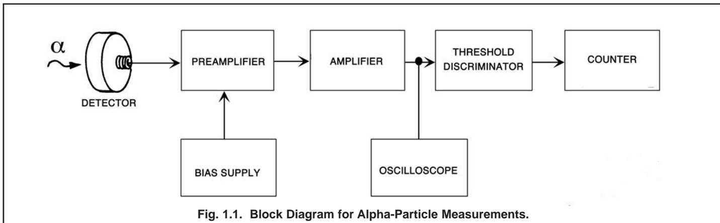
Fig. 1.1. Block Diagram for Alpha-Particle Measurements.
