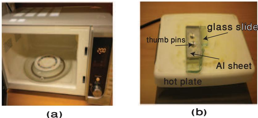
Figure 7: (a) Heat KNO<sub>3</sub> powder in a conventional microwave oven, then (b) melt KNO<sub>3</sub> powder on Al sheet to make thin film with inverted thumbpins acting as electrodes.
