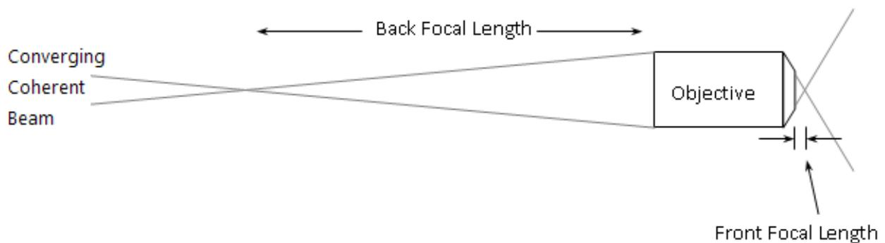
Figure 3. Focal lengths of a microscope objective
