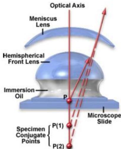
Figure 5. Ray optics for an oil immersion microscope objective.
