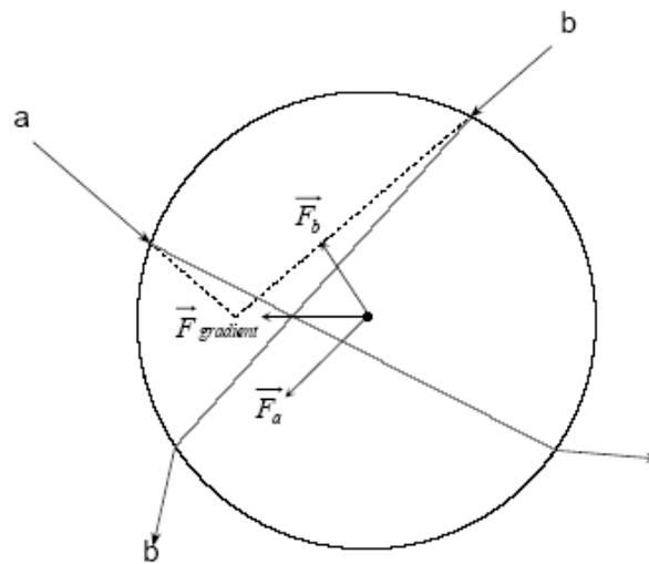
Figure 2. Forces on a trapped bead being pulled to the left.
