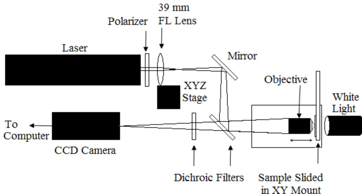
Figure 6. Optics configuration for optical tweezers
