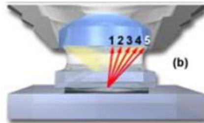
Figure 4. b) an objective with oil as an immersion medium.
