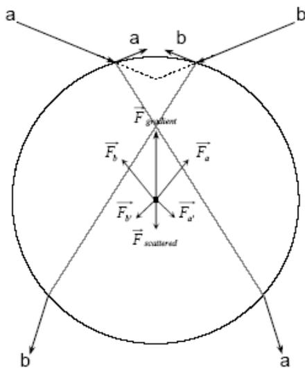
Figure 1. Ray Optics of a trapped bead. A gradient force is created by the refracted rays, while a scattered force is created by the reflected rays.
