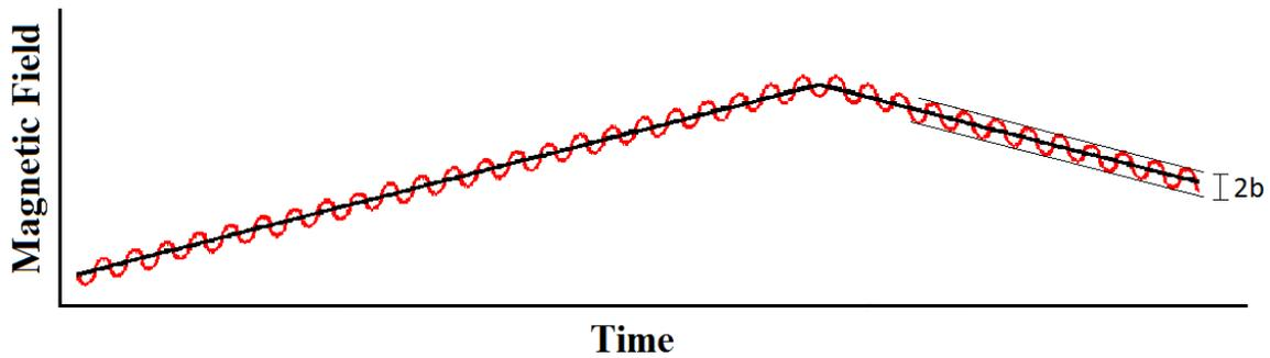
**Figure 4: Effect of modulation on magnetic field strength: The black line represents the field of the main magnet as it is ramped with a triangle wave. The red curve represents the combined field strength of the main magnet and the modulation coils. Note: Not drawn to scale.**
