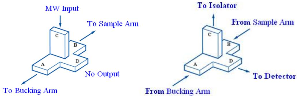
Figure 3B: The Magic T. - How the T in this experiment before and after absorption
