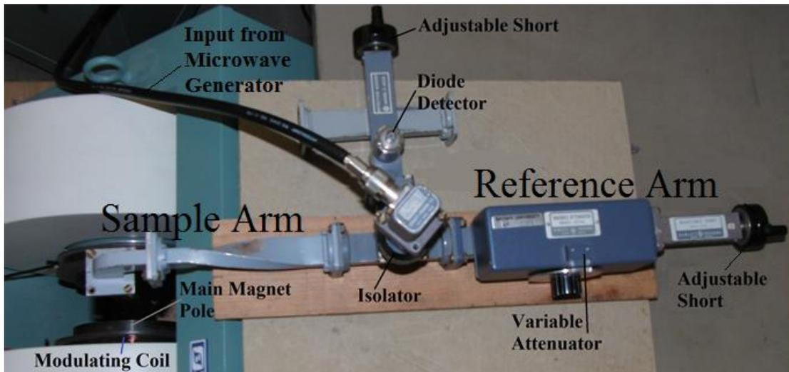
Figure 4: The Spectrometer
