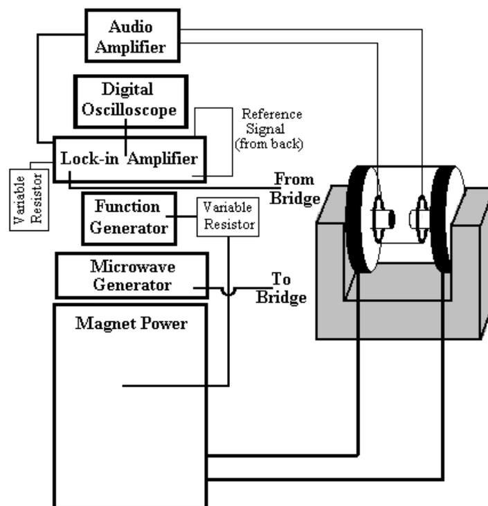
Figure 7: Setup used to observe resonant absorption
