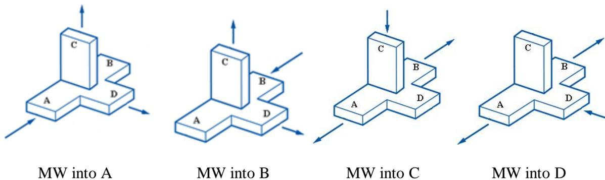
Figure 2A: The Magic T. - Behavior of microwaves entering each of the four arms
