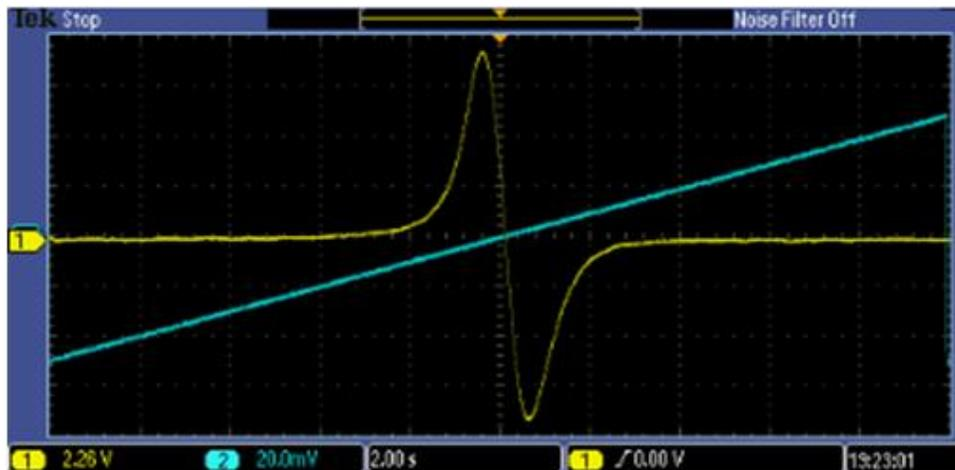
Figure 5: A very nice looking signal. Note the antisymmetry; the signal should ideally have equal weight and width above and below the horizontal axis. The blue line is the function generator sweeping the magnetic field through resonance.
