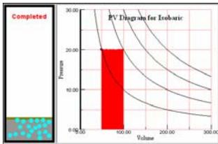
Ideal gas law:  $PV = nRT$ . In this animation  $N = nR$  (i.e.,  $k_B = 1$ ). This, then, gives the ideal gas law as  $PV = NT$ . The work done during a thermodynamic process depends on the type of process (and can be positive, negative, or zero). [Restart](#). Work is given by the equation
