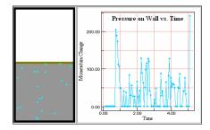
The relationship between the number of particles in a gas, the volume of the container holding the gas, the pressure of the gas, and the temperature of the gas is described by the ideal gas law: PV = nRT. In this animation N = nR (i.e.,  $k_B = 1$ ). This, then, gives the ideal gas law as PV = NT. Restart.
