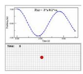
This Exploration allows you to choose initial conditions and forces *with damping*, and then view how that force affects the red ball. You can rightclick on the graph to make a copy at any time. If you check the "strip chart" mode box, the top graph will show data for a time interval that you set. Note that the animation will end when the position of the ball exceeds +/-100 m from the origin. <u>Restart</u>.
