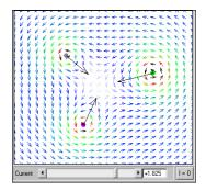
The purple wire and the green wires have fixed currents and fixed positions. You can change the current in the gray wire by using the slider and you can also drag the gray wire around to new positions. The animation shows the magnetic field vectors as well as the force on the wires. You can also add field lines by double-clicking.
