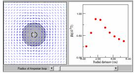
The gray circle in the center represents a cross section of a wire carrying current coming out of the computer screen. The current is uniformly distributed throughout the wire (position is given in centimeters and magnetic field strength is given in millitesla). The black circle is an Amperian loop with a radius you can change with the slider.
