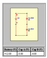
This animation contrasts two configurations of capacitors and a battery **(capacitance is given in farads)**. The table shows the voltage across the battery as well as across each capacitor.
