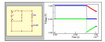
In this animation, you can close and open switches to see what happens to the voltage across the capacitor (red), the voltage across the resistor (green), and the total voltage across the capacitor plus resistor (blue). Initially, the capacitor is charged. After pushing *play*, you should throw the switches (voltage is given in volts and time is given in seconds). <u>Restart</u>.
