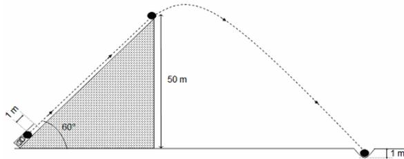
A ball of mass 2 kg is held against a spring compressed by 1 m with a spring constant of  $k = 3 \times 10^3 \text{ N/m}$ , and sits at the bottom of a ramp 50 m high. The ramp is inclined at an angle of  $60^\circ$ . When the ball is released, assuming a frictionless ramp and no wind resistance, the ball will hit a pit of sand. The depth the ball sinks into the sand is 1 m.
