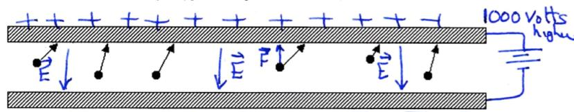
The dust particles are first electrically charged by a small electric discharge and then blown along with the air left to right between the charged plates using a fan. The two plates are wired to a voltage supply so the top plate is 1000 volts higher in voltage than the bottom plate. The two plates are spaced 1 cm apart. The particles are strongly attracted to the top plate and stick there. They can later be removed by just wiping the top plate with a cloth.
