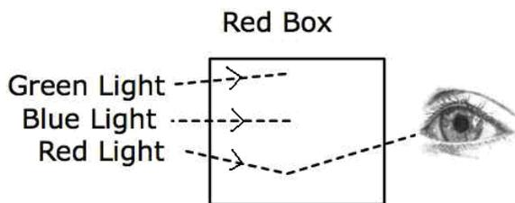
**FIGURE 1.** Opaque model. Green light and blue light are absorbed by a red colored box. Red light is reflected off the red box and seen by the eye.
