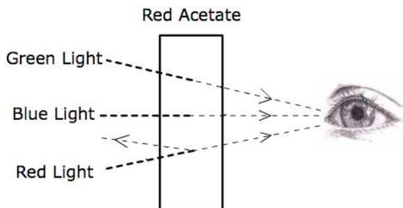
**FIGURE 3.** Compromise model. Some of the green and blue light is absorbed and some is transmitted through. Some red light is reflected back and some is transmitted through. The left side of the model appears to mimic the opaque (red light is reflected and green and blue light is absorbed), while the right side alters the original model by letting light through.
